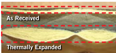
Nomex on Demand is comparable to two or three layers of Nomex E89, but reacts with heat to form a thicker, more insulative structure. Shown is the raw material (top) and the material as incorporated into a liner (bottom).
